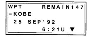
Figure 3-3 Appearance of WPT display after registering a waypoint
